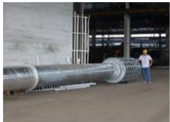
Right: one of the sea water intakes
